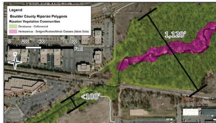
FIGURE 4. EXAMPLE OF VARYING RIPARIAN ZONE WIDTHS THROUGH THE PROJECT AREA. THE NARROW RIPARIAN ZONE (LEFT) IS LIMITED BY LAND USE AND BISECTED BY A RAILROAD; THE MORE NATURALIZED DOWNSTREAM SECTION (RIGHT) IS WIDE AND LESS CONFINED. (NOTE: EXAMPLE IS PROVIDED FOR RIPARIAN WIDTH CHARACTERISTICS ONLY - SITE SPECIFIC VEGETATION COMMUNITIES AND SPECIES MAY NOT REPRESENT AN APPROPRIATE RESTORATION TARGET.)
