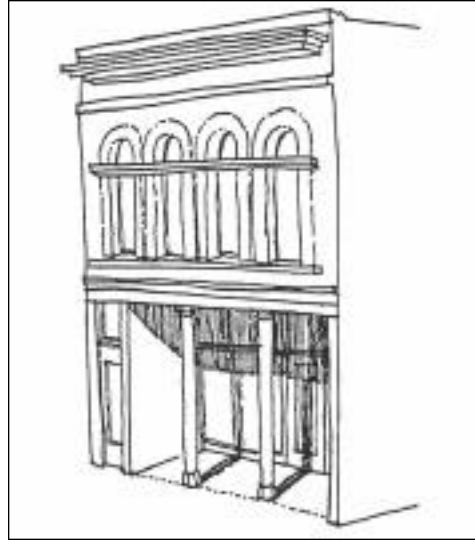
Recessed storefront with columns at sidewalk line
