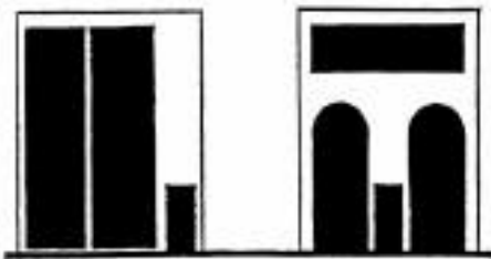
Unacceptable: does not distinguish between upper and lower floors
