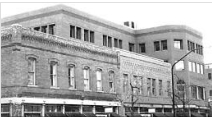
Examples of setbacks on upper floors that reduce perceived height, mass, and scale of buildings.
