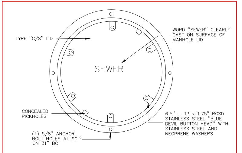
NOTE: STANDARD FRAME AND COVER FOR MANHOLE LOCATED OUTSIDE DEDICATED STREET ROW AND WHERE SURFACE RUNOFF CANNOT BE AVOIDED.
