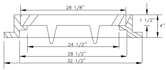
NEENAH PRESSURE TYPE ROUND MH FRAME, C/S BOLTED LID R-6462-GH OR APPROVED EQUAL (SUBMIT TO CITY FOR APPROVAL)
