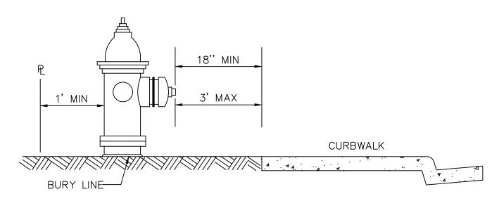
NOTE: FOR FIRE HYDRANT INSTALLATION, SEE DETAIL DRAWING NO. 5.13.
