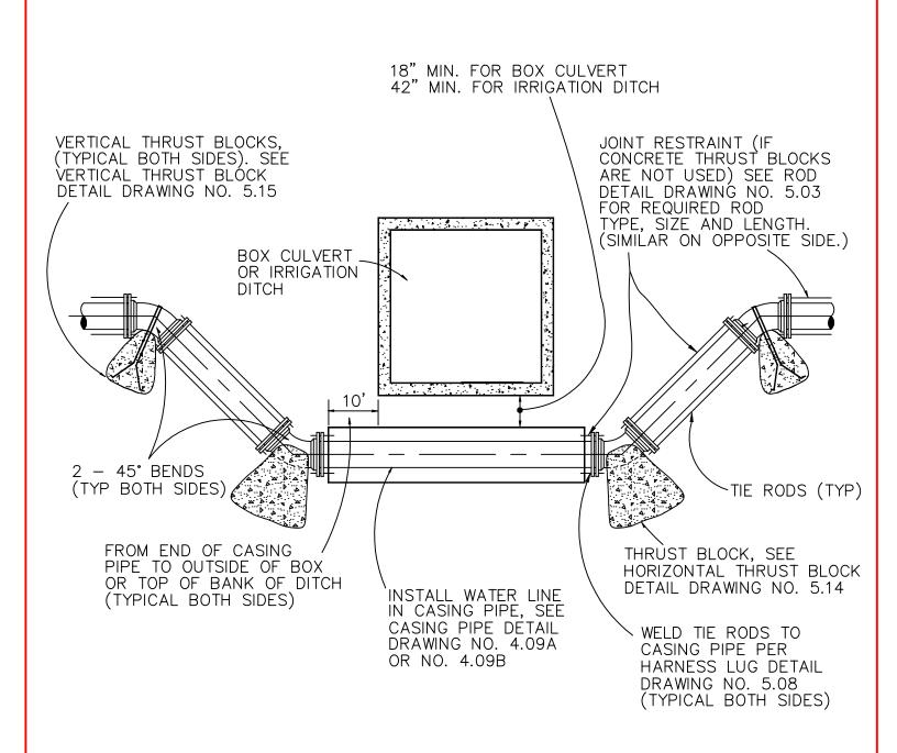
NOTE: PIPE RESTRAINT SHALL BE EITHER CONCRETE THRUST BLOCKS OR JOINT RESTRAINT AS SPECIFIED.
