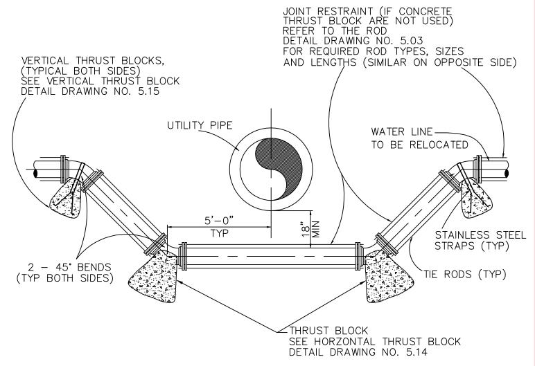
NOTE: PIPE RESTRAINT SHALL BE EITHER CONCRETE THRUST BLOCKS OR JOINT RESTRAINT AS SPECIFIED
