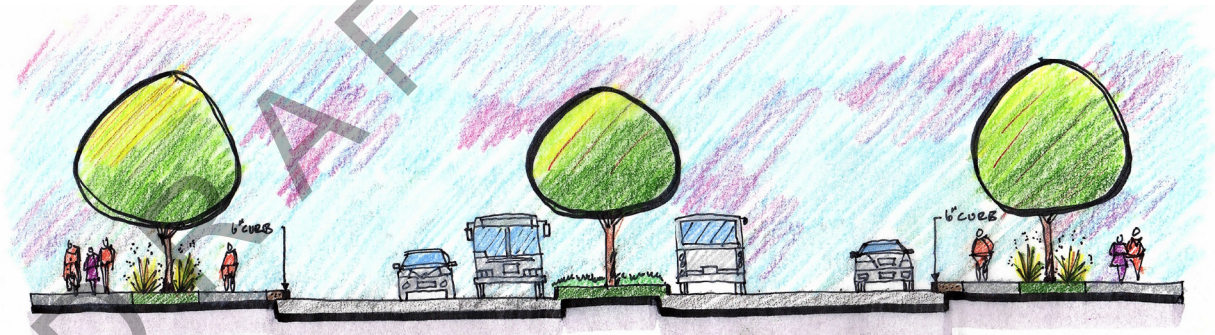
CENTER-RUNNING BRT - EXAMPLE CROSS-SECTION
