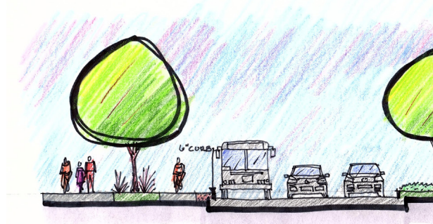
CURBSIDE RAISED PROTECTED BICYCLE LANE Separated from the sidewalk/multi-use path by an amenity zone. (Example cross section - Option 1)
