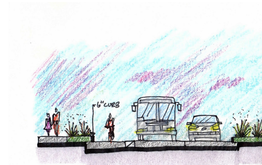
STREET-LEVEL BUFFERED BICYCLE LANE Separated from travel lanes by a striped buffer. (Example cross section - Option 4)
