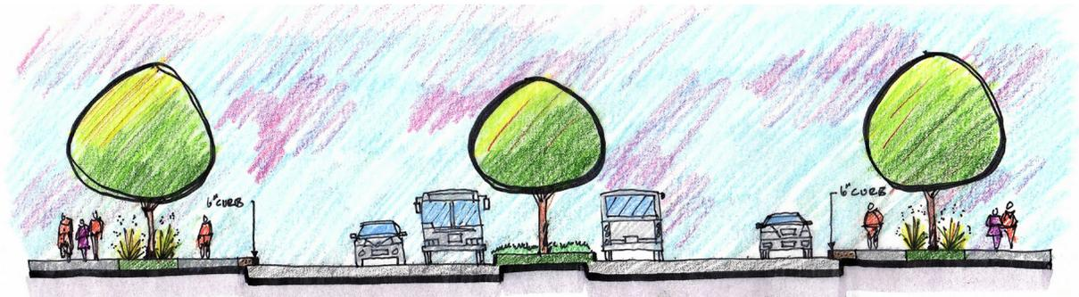
CENTER-RUNNING BRT - EXAMPLE CROSS-SECTION
